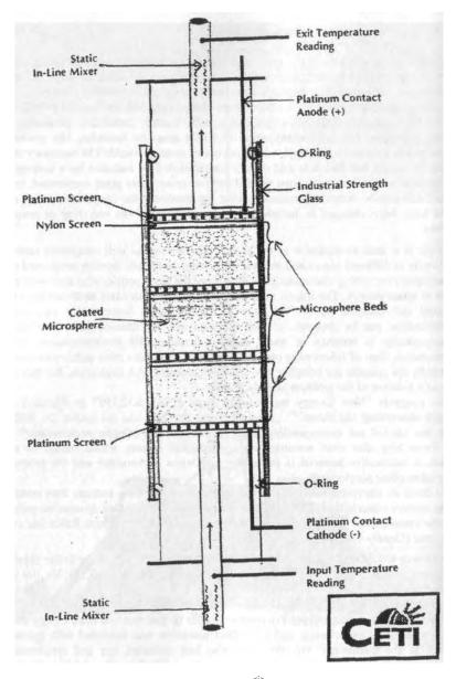
Fig. 17.4: 1 kW Patterson Power Cell.
