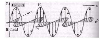
Fig. 21.8 B: The planar electromagnetic wave in the proximity
