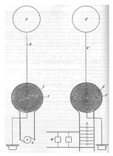
Fig. 9.7: Wireless energy transmission, Patent No. 645,576 (1900) of Testa.<sup><i></sup>
