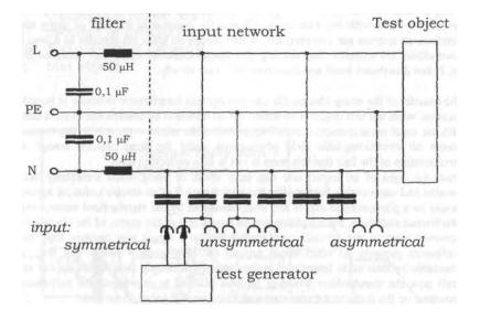
Fig. 2.6: Picking up of interference voltages in network lines.<sup><i></sup>
