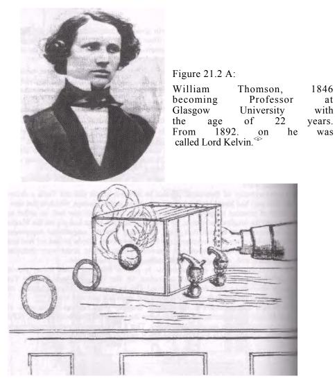
Fig. 21.2 B: Vortex rings from a smoke vortex gun.<sup><i></sup>
