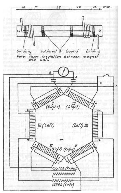
Fig. 16.8 C: The Coler converter
