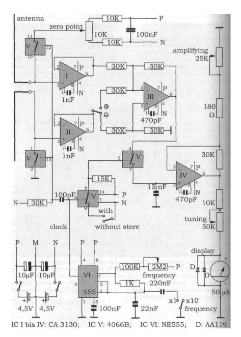
Fig. 19.2: Wiring diagram of the self-built charge amplifier
