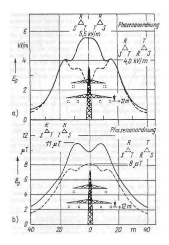
profile of the 50-Hz-field on the ground at 380 kV/1 kA in each circuit.<sup><i></sup> Fig. 2. 11: a) electric field,
