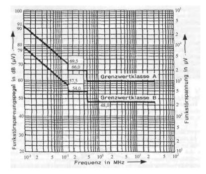
Fig. 2.2: Classes of limits according to VDE 0871(since 1-1-96: VDE 0875)<sup><i></sup>
