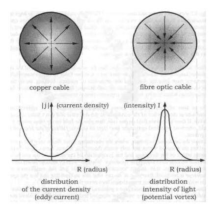
Fig. 4.1: The distribution in principle of the intensity of light within a fibre optic  $cable^{<i>}$  compared to the
