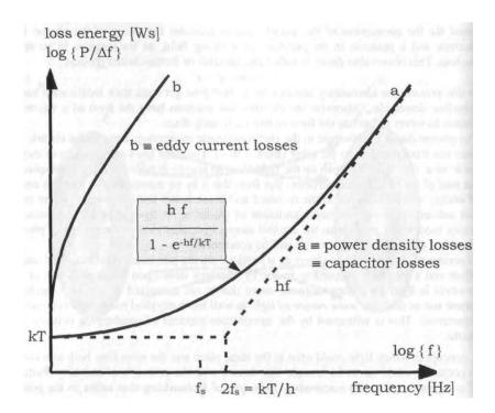
Fig. 4.7: The power density shown against frequency for noise
