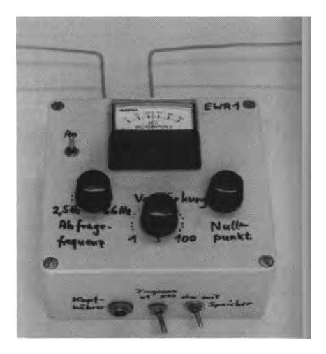
Fig. 19.1: A self-built charge amplifier.
