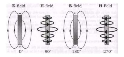
Fig. 21.8 A: The fields of the oscillating dipole antenna.<sup><i></sup>
