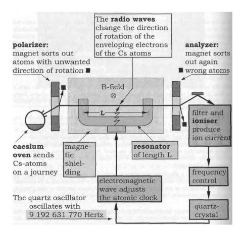
Schematic representation concerning principle of functioning L =length of resonator determining the exactness
