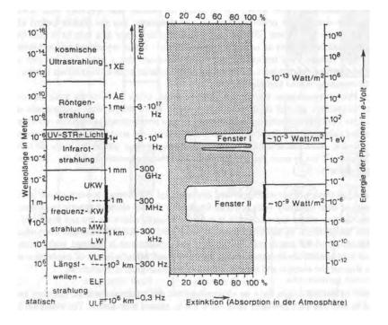
Fig. 2.8: Absorption dependent on frequency in the atmosphere
