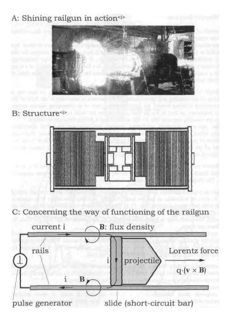
Fig. 15.5: Structure and way of functioning of the railgun
