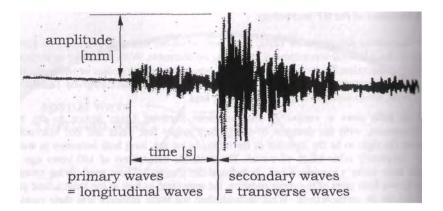
Fig. 21.7 A: Longitudinal and transverse earth quake waves.
