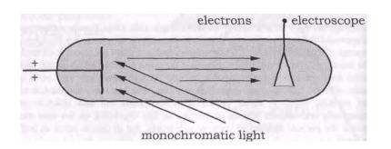
Fig. 22.2 B: The photo-electric effect
