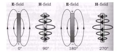
Fig. 21.8 A: The fields of the oscillating dipole antenna
