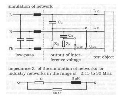
Fig. 2.4: Simulation of network for the measurement of interference voltages.  $\leq >$
