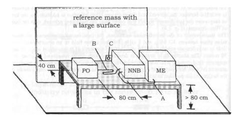
Fig. 2.5: Measurement set up to measure the emission of interferences bound to a conductor,  $\overset{<i>}{}$
