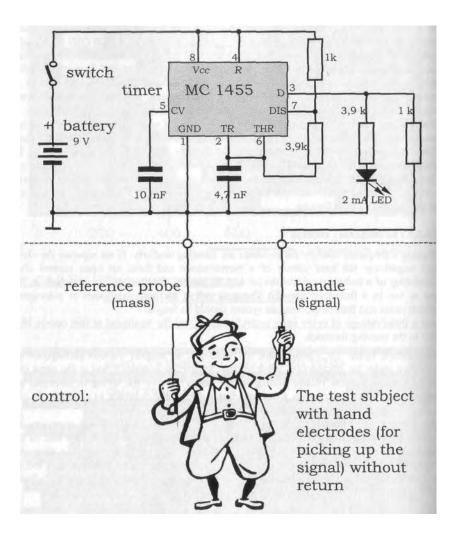
Fig. 24.4: Wiring diagram of the Zapper.<sup><i></sup>
