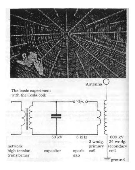
Fig. 9.1: High tension transmitter of Nikola Tesla
