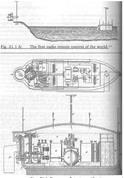
Fig. 21.1 B: Patent specification concerning the remote controlled submarine.<sup><i></sup>
