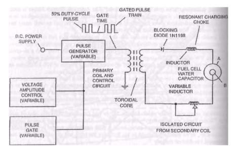
Fig. 17.7: Wiring diagram for the driving of the water-cell<sup><i></sup>
