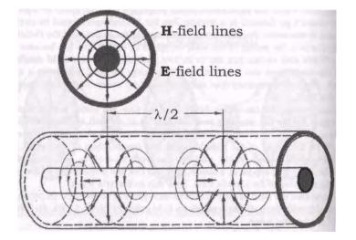
Figure 21.11 B: Wave propagation in a coaxial cable, (Example for waveguide, horn radiator, etc.)<sup><i></sup> Cross-section of coaxial conductor and field distribution in the direction of propagation.
