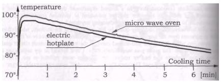
Fig. 19.7: Measurement curve of the water temperature over time
