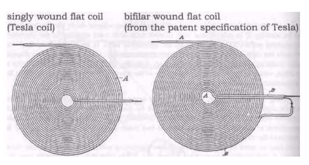
Fig. 16.9 A: Coiling techniques of Tesla's flat coil.
