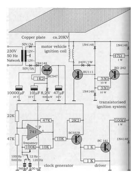
Fig. 19.4: Wiring diagram concerning the Kirlian device.<i>
