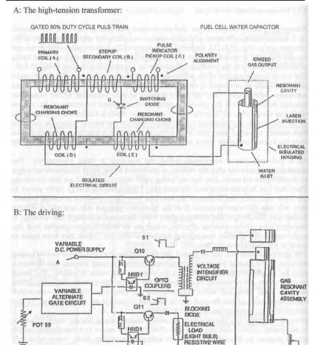
Fig. 17.8: High-tension transformer and driving of the cylindrical water-cell<i>
