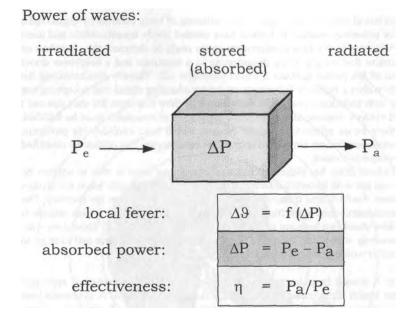
Fig. 1.3: Damping of waves and ability to absorb of a body (our head) if we are making a phone call with a handy.
